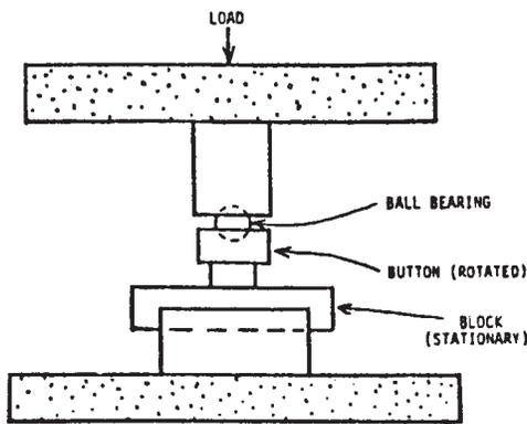
FIG. 2 Schematic Diagram of Galling Test Set-Up
