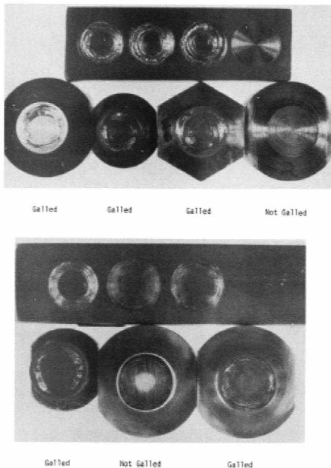
**FIG. 4 Test Specimens**
